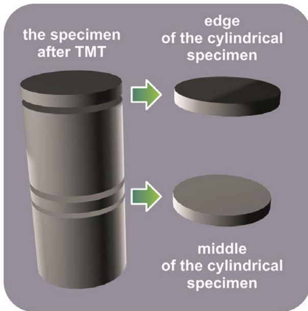
Fig. 1. Scheme of cutting samples for investigation
