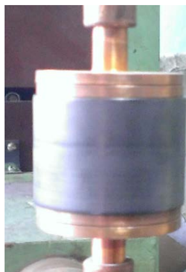
Fig. 6. Accessories for electric current assisted sintering in the spot welding machine
