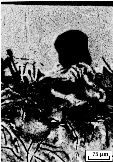
Fig.2 Incompleteness due to partial evaporation of graphite inclusion at the bottom of the molten bath in GG 15 upon laser treatment with the following parameters: N_s=1.9 \cdot 10^4 w/cm 2 , E_v=1.58 \cdot 10^4 J/cm 3 .
