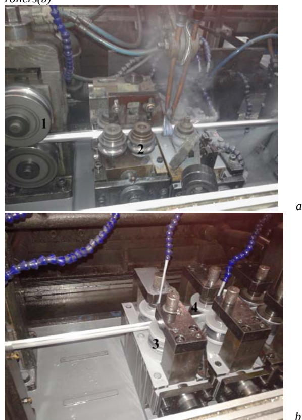
Fig.6: Section rolling machine for aluminum profiles: 1, 2, 3, 4 – rollers in the work
