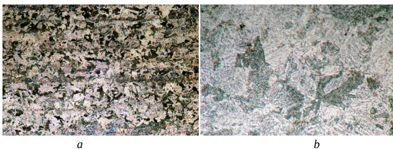
Figure 5 (a and b) Microstructure of initial material, Villela reagent a. \times 100 b. \times 200
