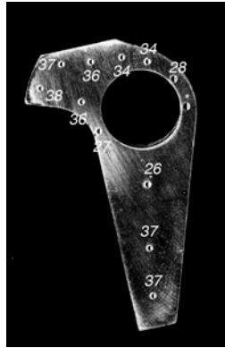
Figure 1 (a - c) Metallographic specimen and measured hardness values according Rockvel and Vickers method
