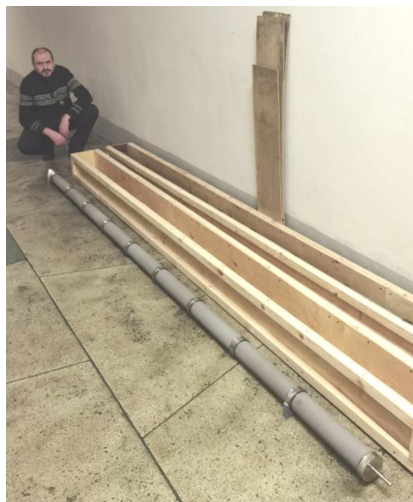
Fig. 5. Titanium filter element for filtering gaseous melamine.
